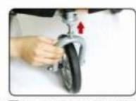
the slot till hearing the spring clip click. Check the front wheel is securely locked by pulling. (Skip this step if you are going to use it as a bicycle trailer)
