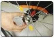
Push rear wheel to the bottom 3 of axle till the spring clip clicks. Check both wheels are securely locked by pulling.
